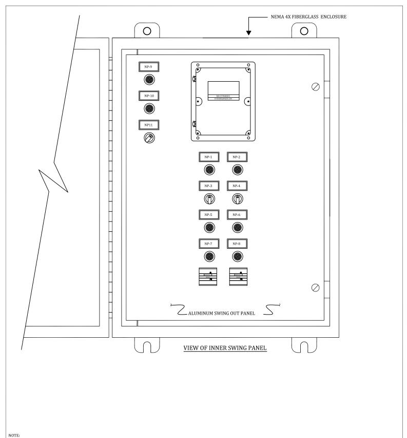
NOTE: SEWER GASSES WILL DESTROY COMPONENTS IN PANEL. PROPER SEALS MUST BE INSTALLED EXTERNAL TO THE PANEL TO PREVENT ENTRY OF GASSES.
