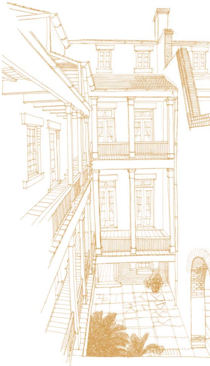
Courtyards provide ventilation, outdoor living space, and garden space within urban environments. Galleries often line the interior of the courtyard and provide shade for the building. (Sketch by John Desmond, FAIA)
